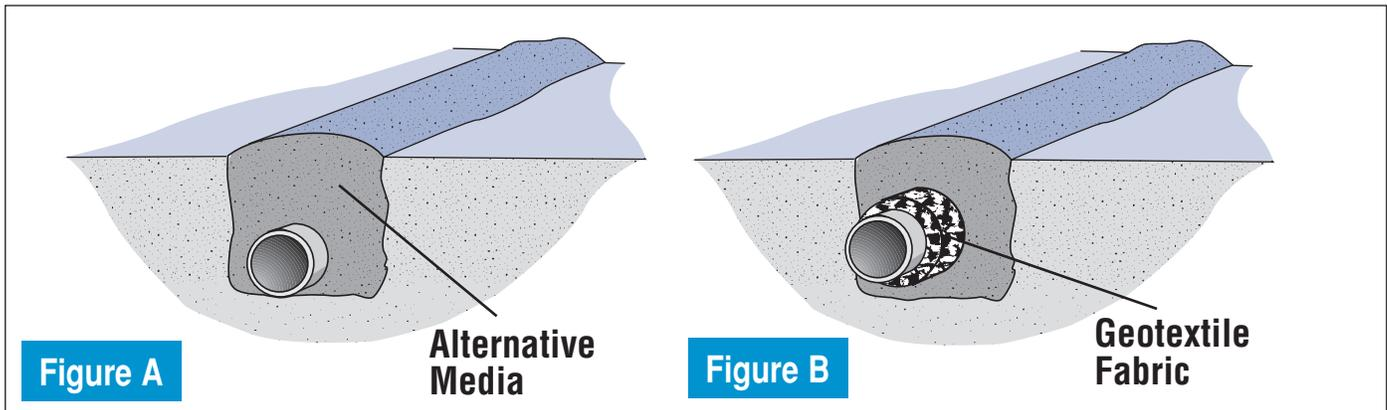
• **Easier on Soils**—Gravelless systems may be a good choice in areas that have soils susceptible to “smearing” or other structural damage. Soil structure can be impacted by the weight of gravel itself or by construction and heavy machinery on the site.
