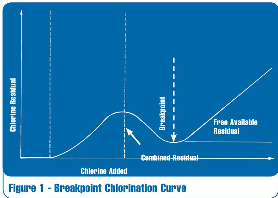
Figure 1 - Breakpoint Chlorination Curve
