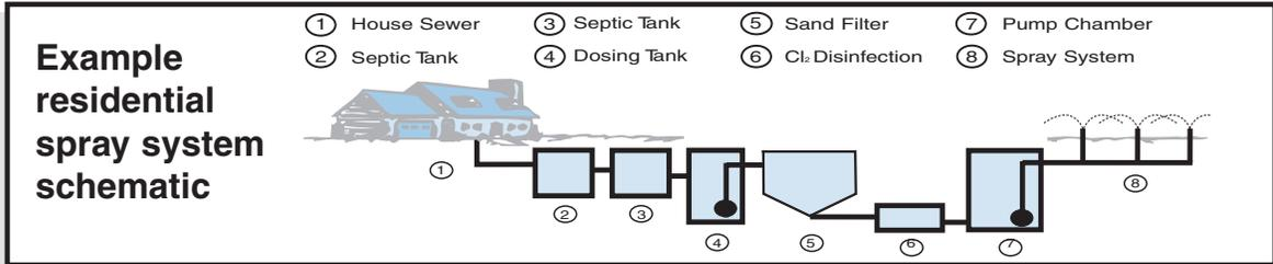
Spray irrigation is an efficient way to nourish plants and apply reclaimed wastewater to land. Some spray systems are very similar to potable-water sprinkler systems used to irrigate lawns. Others are specifically designed for agricultural applications.
