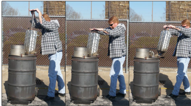
1-2-3... Mark Kruger injects bottles of prescription medication into the Bella Vista, Arkansas, Police Department's Drug Incinerator. The incinerator is used as an alternative to flushing unwanted drugs, which can make their way into the drinking water system.
