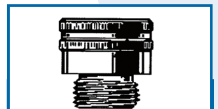
A typical screw-on vacuum breaker for a hose bib.
