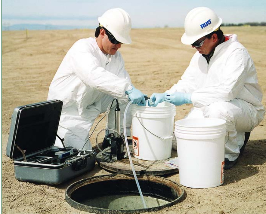
Using a groundwater remediation system, the U.S. Army Corps of Engineers do some sampling to check the water quality at the Pueblo Depot in Pueblo, Colorado.
