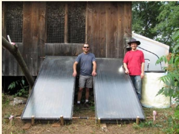
*The Rich Earth Institute has experimented with solar pasteurizers to reduce the amount of storage time needed to sanitize the urine. The pictured unit was designed to sanitize 50 gallons of urine by heating it to 70° C (158° F) for 30 minutes.*
