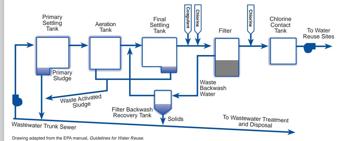
Drawing adapted from the EPA manual, *Guidelines for Water Reuse*.
