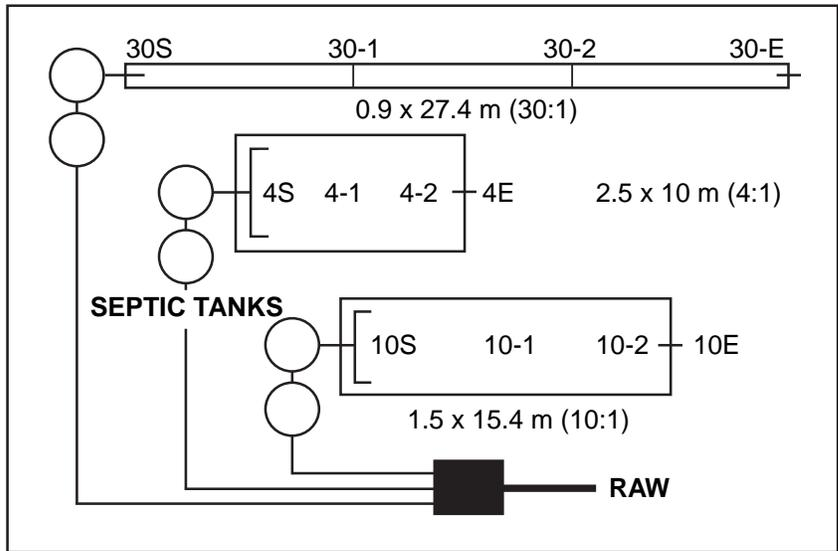
**FIGURE 2** ▲ Plan view of experimental facility showing sampling ports for septic tank effluent (not to scale).
