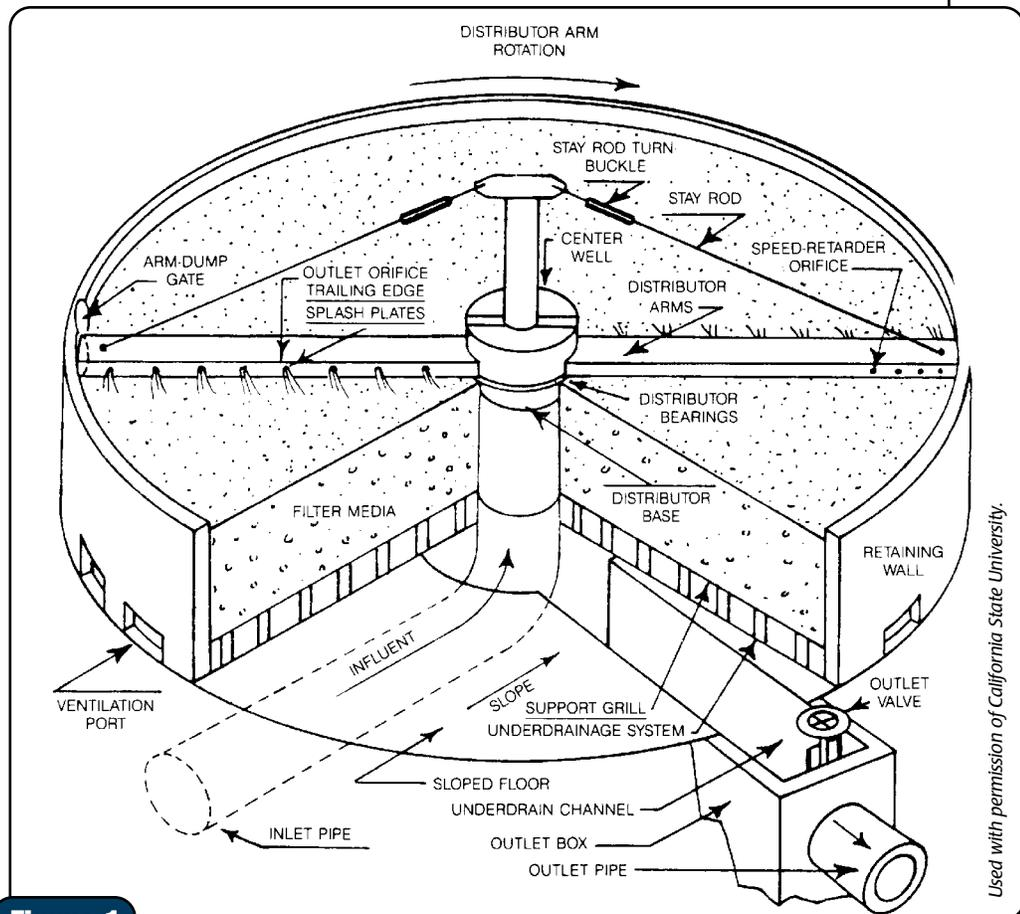
**Figure 1** Parts of a typical trickling filter.
