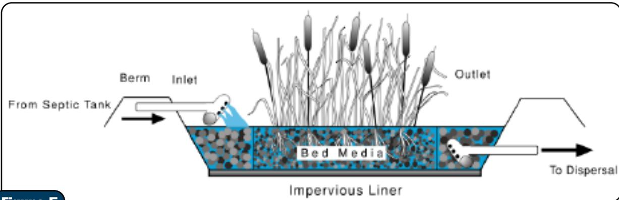
**Figure 5** Constructed Wetland
