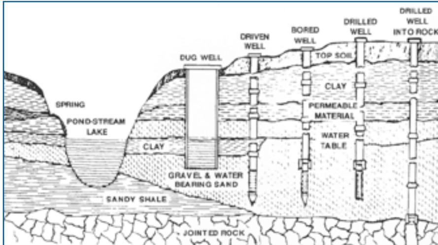
Typical cross-section of underground strata, showing various types of well construction
