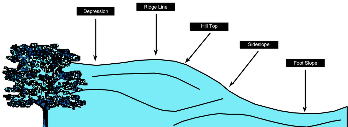
**FIGURE 2** Landscape contours help estimate surface and subsurface drainage patterns. Hilltops and side slopes drain well, whereas depressions and foot slopes drain poorly.
