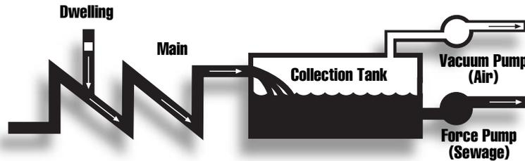
Usually three- or four-inch diameter pipes from the service connection and four- to 10-inch mains are used for vacuum systems, depending on the flow and design of the system.
