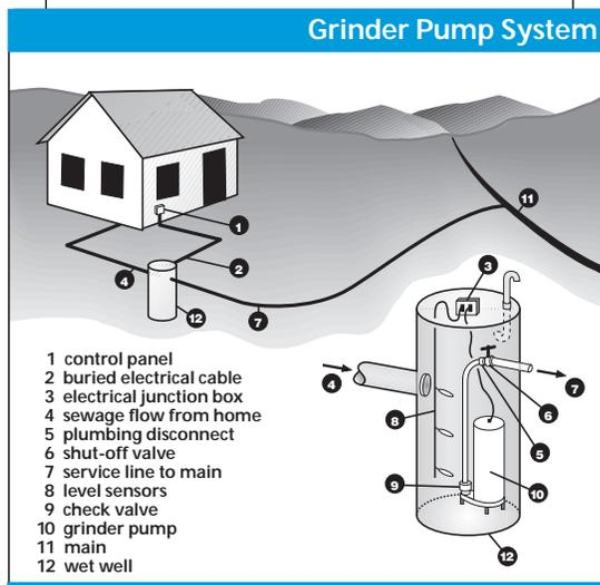
to the tank. The effluent enters the pumping chamber and triggers a sensor when it rises to a certain level. The effluent is then pumped out for a few minutes until the water level is reduced and a lower level sensor shuts the pump off. There is also a sensor that triggers an alarm if, for some reason, effluent levels get too high in the pumping chamber.
