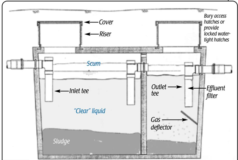
**Figure 1** Diagram of a typical dual compartment tank.
