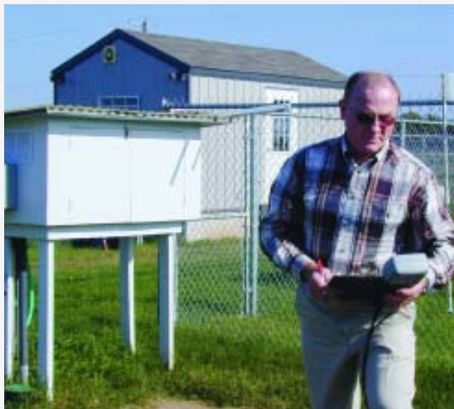
Dissolved oxygen, pH, and temperature readings are taken in-situ.
