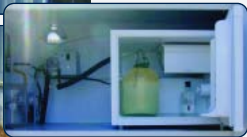
Close-up of a sample enclosure in a refrigerator. The peristaltic pump and sample timer are to the left.
