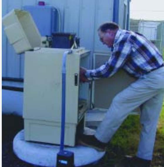
Jumper checking the composited raw wastewater sample in the Isco refrigerated sampler.
